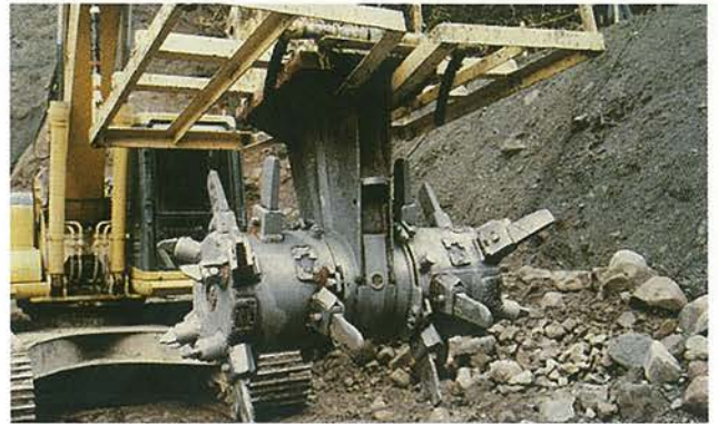
■ Twin header attached to the backhoe
